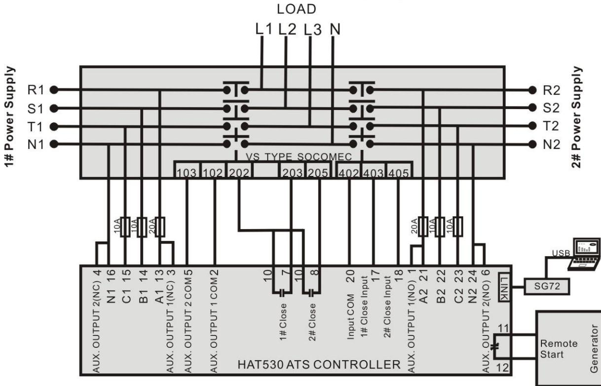
**Note:** The diagram is for reference only. The actual wiring shall follow the ATS instruction. Users should choose proper fuse capacity according to the actual power consumption. If SOCOMECS VS is applied, the Close delay and Open delay must be no less than 5s (Default: 5s).
