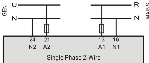
**NOTE:** Above pictures take the AC 220V voltage as example. If AC 110V voltage is applied in actual use, please contact with Smartgen technical staff to get the specific wiring methods.
