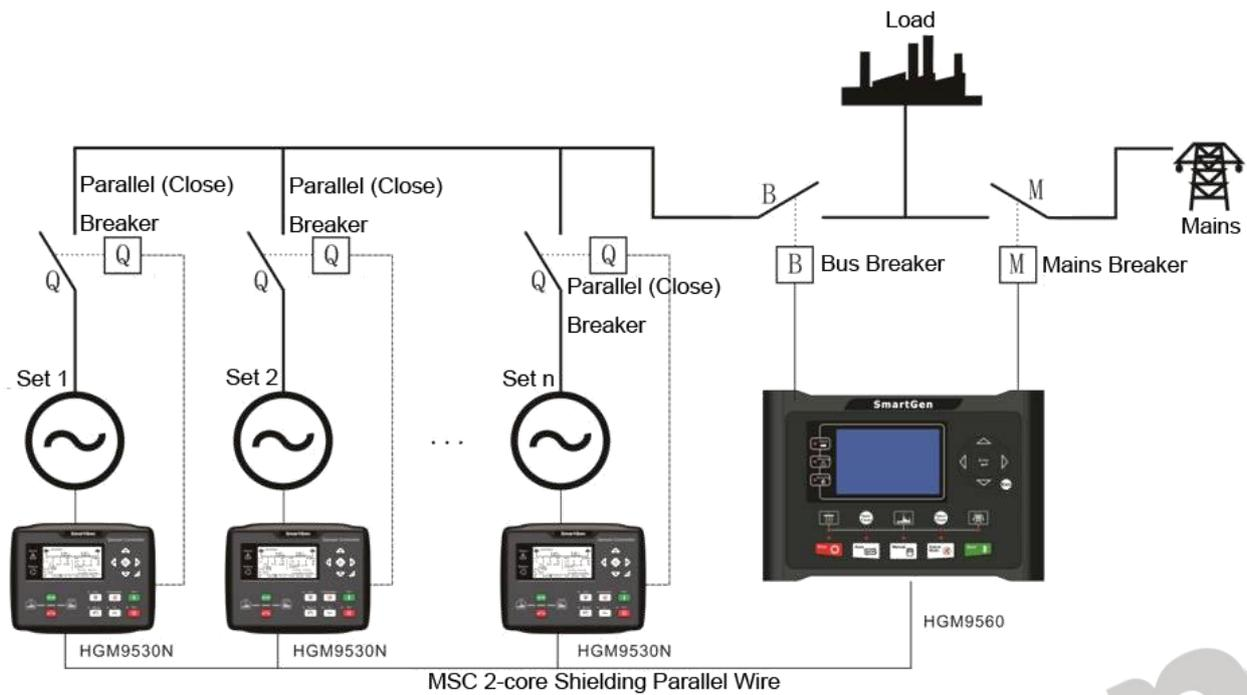
**Fig. 9 HGM9510N/9530N Multi-genset Parallel Application Graph**
